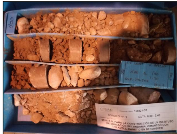
Figura 1. Testigo sondeo 1 (0.00 a 2.40 m)
